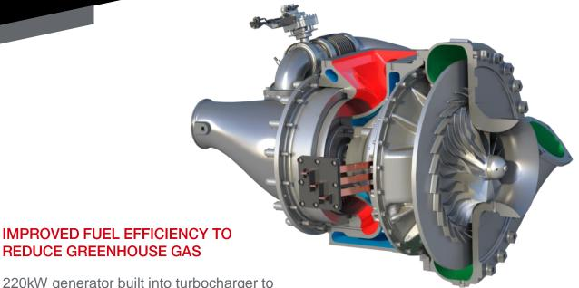
220kW generator built into turbocharger to power traction motor #3 and reduce fuel consumption on High Pressure Common Rail EVO engines.
